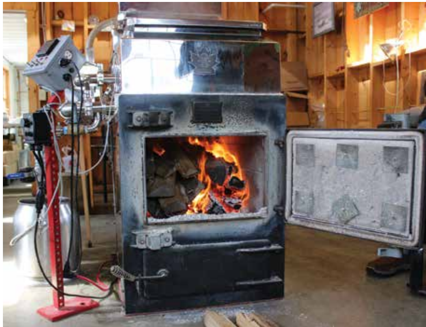
This firewood operated evaporator helps with the sugaring process.
